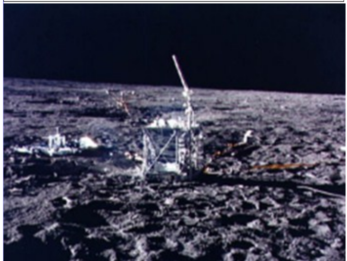
The seismic station at the Apollo 12 site. The seismometer monitors the level of ground motion to detect arriving seismic waves. The instrument (left) is protected by metal foil against the varying temperatures on the lunar surface that produce large thermal stresses. Credit: NASA
